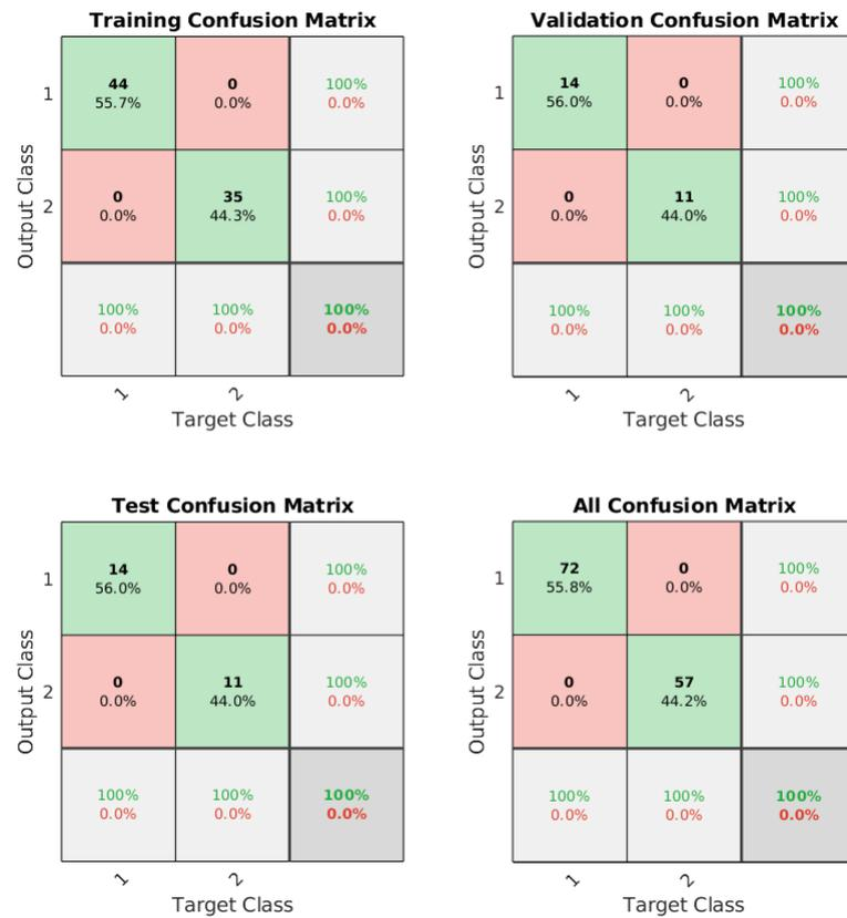
Figure 5.14. Confusion graph of a low and high bacteria concentration classification experiment on minute 4 samples with ANN structure of a single hidden layer with 5 neurons. Perfect result is obtained with PCA, LDAP and first PCA then LDA approaches.
