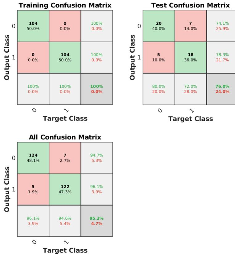
Figure 5.15. Confusion graph of a with and without bacteria solution classification experiment by applying PCA on minute 4 samples with SVM
