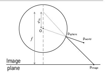
Fig. 3: In the spherical camera model, a point is projected onto the unit sphere first, then projected onto the image plane. For cameras using parabolic mirrors,  $\xi = 1$ .
