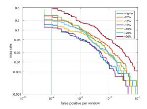
Fig. 7: The performance of the proposed method (RICF) on the INRIA dataset, where each window is transformed into an omnidirectional image. The performance decreases rapidly as the test images gets further away from the camera. Best viewed in color.
