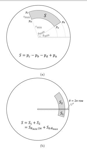
Fig. 4: (a) Illustration of rapid computation of the sum inside an annular region using radial integral image. Four look-ups and three operations are sufficient to calculate the sum. (b) If an annular sector query crosses  $\theta = 2\pi$  angle, it can be broken up into two annular sectors. In this case, an extra column is needed to look-up values that correspond to  $\theta = 2\pi$ .
