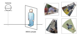
Fig. 6: Left: Each sample in the INRIA dataset is placed on the ground plane and a virtual omnidirectional image is formed (camera is shown as a sphere since we used the sphere camera model). Right: Some examples of the resulting images.
