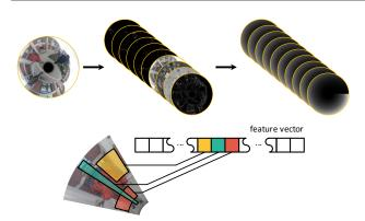
Fig. 2: Visualization of the radial integral channel features. Top: First, the input image is transformed into various channels (LUV, gradient magnitude etc). Then, radial integral images are formed. Bottom: Lastly, for a given annular sector shaped window, the sum inside the annular sectors (corresponding to a channel) is calculated. Features are shown on the original image for clarity.
