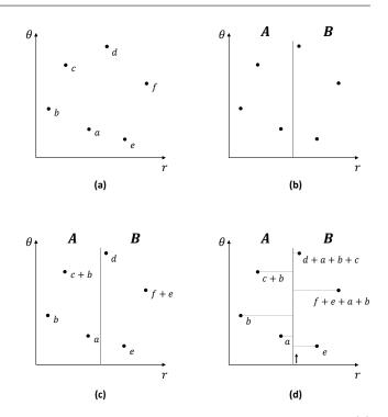
Fig. 5: Steps of computing the radial integral image. (a) Polar coordinates and values of the pixel are given as the input. (b) Pixels are split from the median radius to form two equally sized sets, A and B. (c) The algorithm is recursively called for each set. (d) Pixels are iterated according to increasing angle value and two sets are merged by updating the values in B.
