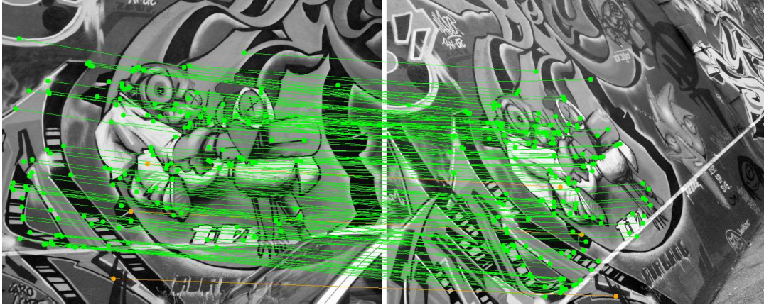
Figure 2.4. Outputs of Outlier Filtering: Outlier filtering, or geometric verification, involves determining the transformation parameters that have the largest consensus among the provided point correspondences. The most popular algorithm for performing this task is Random Sample Consensus (RANSAC). The RANSAC algorithm is used to reject outliers among the matches. In its simplest form, RANSAC randomly samples a minimal subset of matches to estimate the transformation parameters, which in this case requires 4 point correspondences since they produce 8 equations to estimate 8 parameters. Then, all matches that are sufficiently consistent with the parameters suggested by the minimal subset are counted. This process is repeated many times, and the minimal subset with the best support (highest count) is chosen as the best hypothesis. Matches inconsistent with this best hypothesis are then eliminated. RANSAC has many variants that improve upon its basic components.
