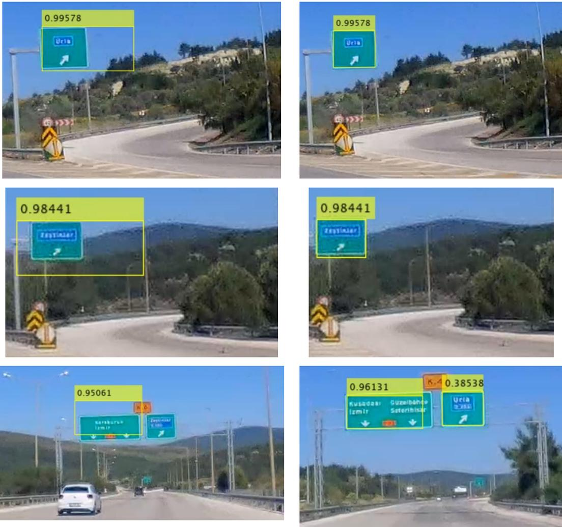
Figure 42. Localizations (left) can be improved (right) by a hybrid approach
