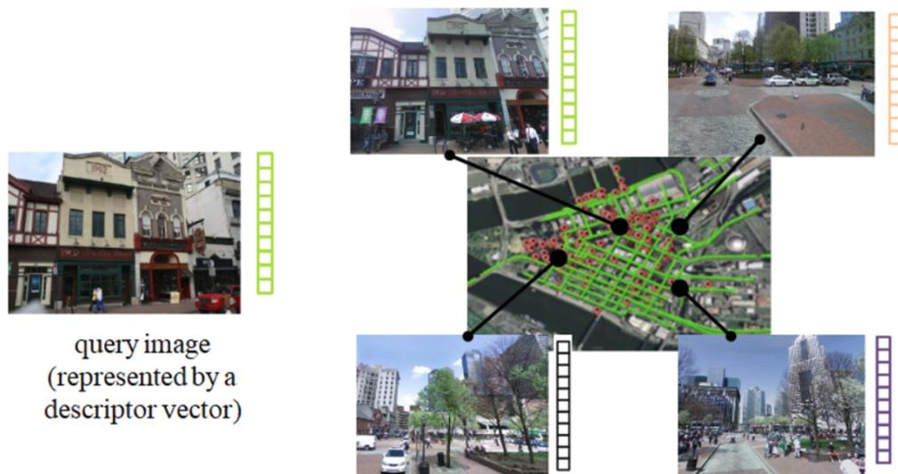
Figure 2.1. On the left, we see a query image. On the right, we see a district with a database of images with known GPS coordinates. Retrieval from the database is based on the similarity of descriptor vectors. The GPS location of the image retrieved from the database serves as the position estimate of the query image. If a correct match is retrieved, then the localization is successful.
