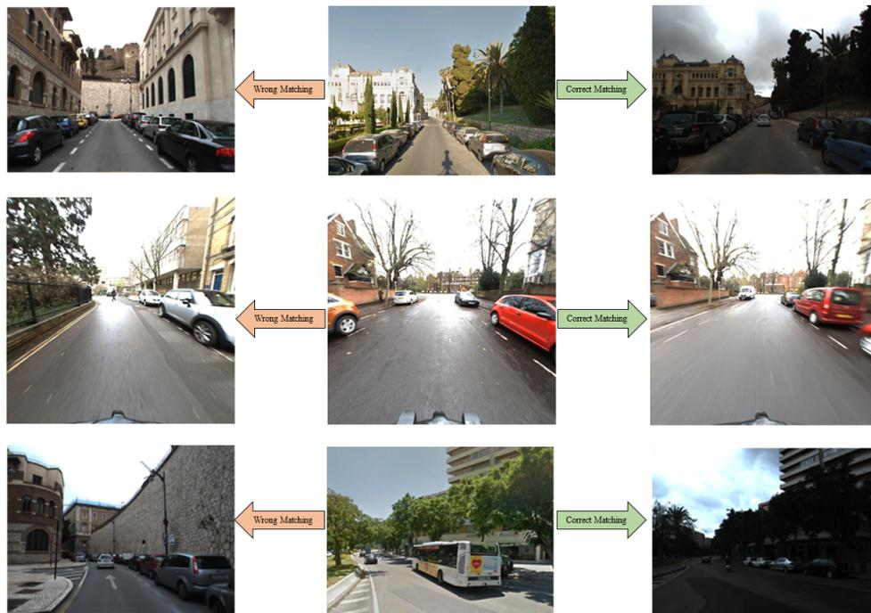
Figure 4.8. Superiority of proposed Hybrid- $VL_{DL}$  method with three sample localization cases from both data sets. RGB image based method  $LD-VL_{NetVLAD}$  (left) fails but Hybrid- $VL_{DL}$  (right) accomplishes for a given query (middle)
