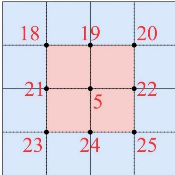
Figure 3.4 The center of the base search window (5), the center points of intersected search windows (18, 19, 20, 21, 22, 23, 24, 25) are away from the center of the base search window by 50 % of the height/width.
