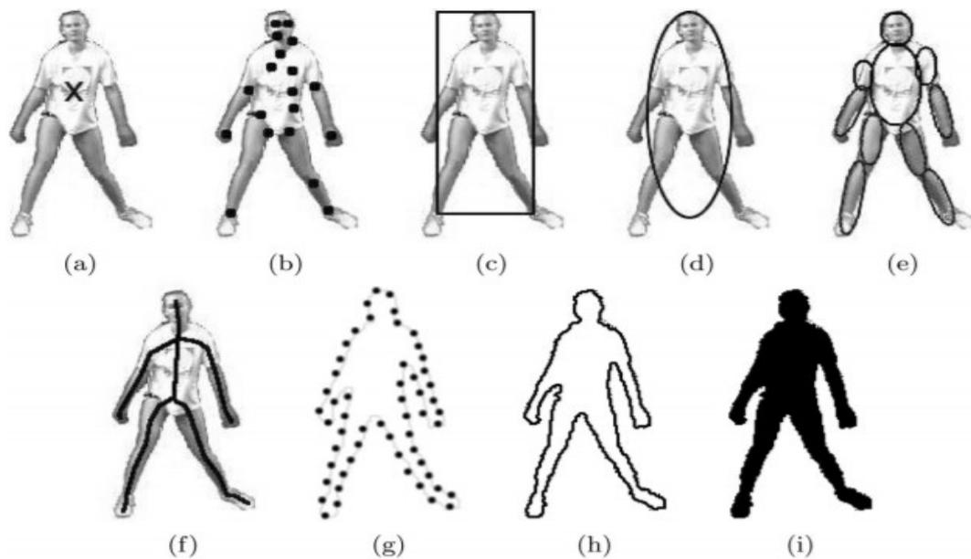
Figure 1.2 Object representations [2] (a) centroid, (b) multiple points, (c) rectangular patch, (d) elliptical patch, (e) part-based multiple patches, (f) object skeleton, (g) complete object contour, (h) control points on object contour, (i) object silhouette
