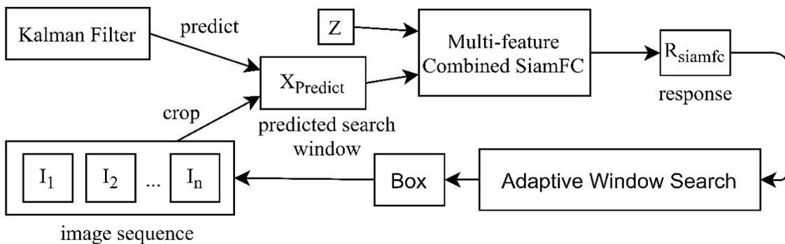
Figure 3.1 The architecture of the proposed Adaptive-Kalman-Siam tracker
