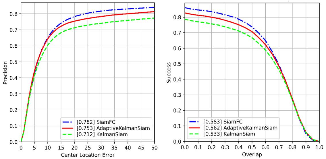
Figure 5.1 The precision and success plot of SiamFC, Kalman-Siam, and Adaptive Kalman-Siam on the OTB-100 dataset using OPE strategy
