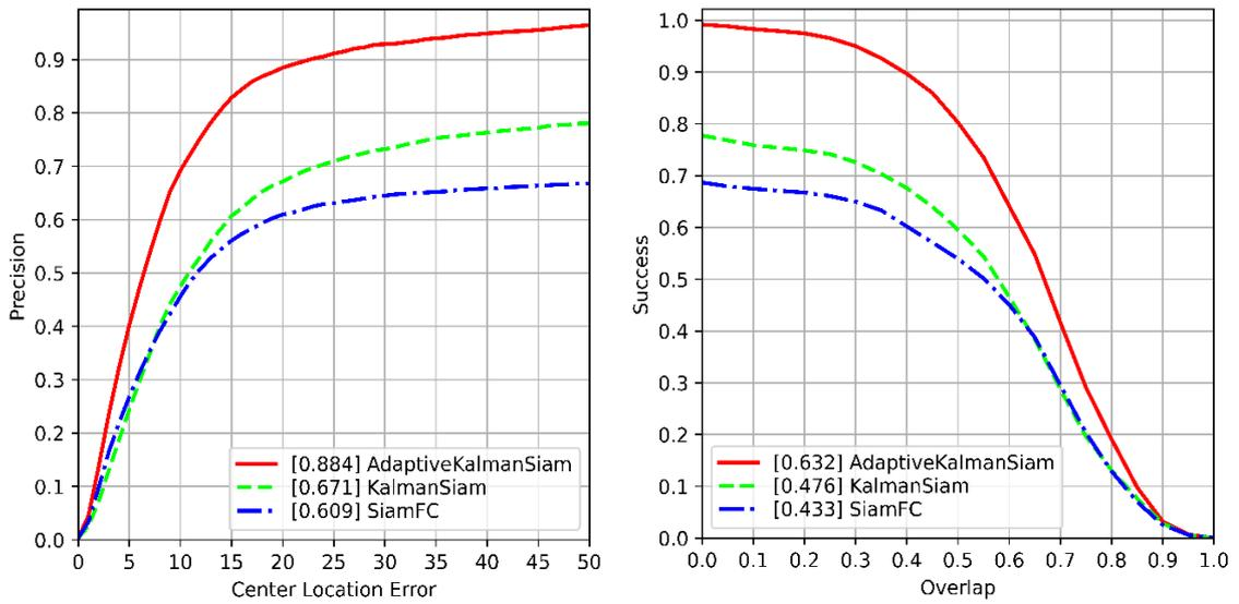
Figure 5.4 The precision and success plots of SiamFC, Kalman-Siam, and Adaptive Kalman-Siam on the IZTECH15-TC dataset using OPE strategy
