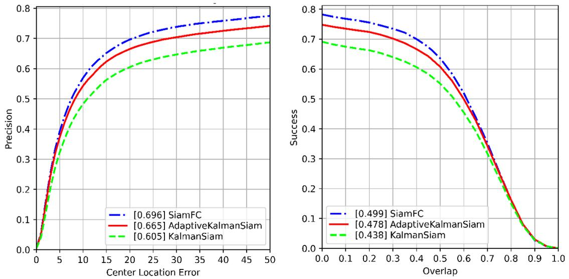
Figure 5.2 The precision and success plots of SiamFC, Kalman-Siam, and Adaptive Kalman-Siam on the TC-128 dataset using OPE strategy
