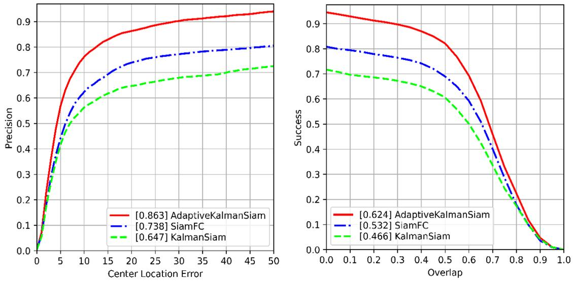
Figure 5.3 The precision and success plots of SiamFC, Kalman-Siam, and Adaptive Kalman-Siam on the IZTECH15-OTB dataset using OPE strategy
