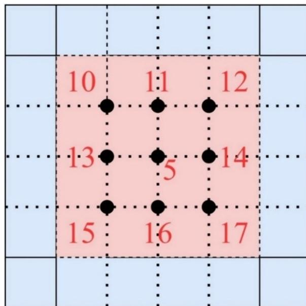
Figure 3.5 The center of the base search window (5), The center points of intersected search windows (10, 11, 12, 13, 14, 15, 16, 17) are away from the center of the base search window by 25% of the height/width.
